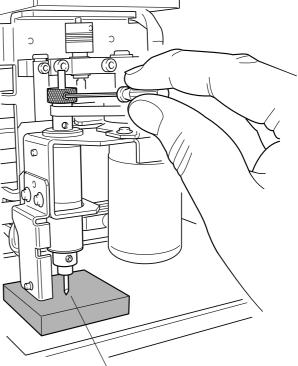
illuminated, then press and hold the Origin Set button for a short while (0.3 second or more). (Pressing the Origin Set button lights the Origin Set light. Make sure the light is illuminated, then release the
